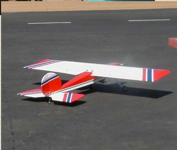
Bill Hill is a busy guy. He has just put together a new plane with a parachute jumper for the Fun Fly. It is a Stick 40 electric ARF. He uses a Spectrum receiver with Hi-Tec 225 servos, Sim prop 28x40 geared 4.4 to 1 with a 13x6.5 prop, 450 watts. It weighs 4 lbs. 6 oz. Test run went very well from take-off to delivery with accurate drops & recoveries.
