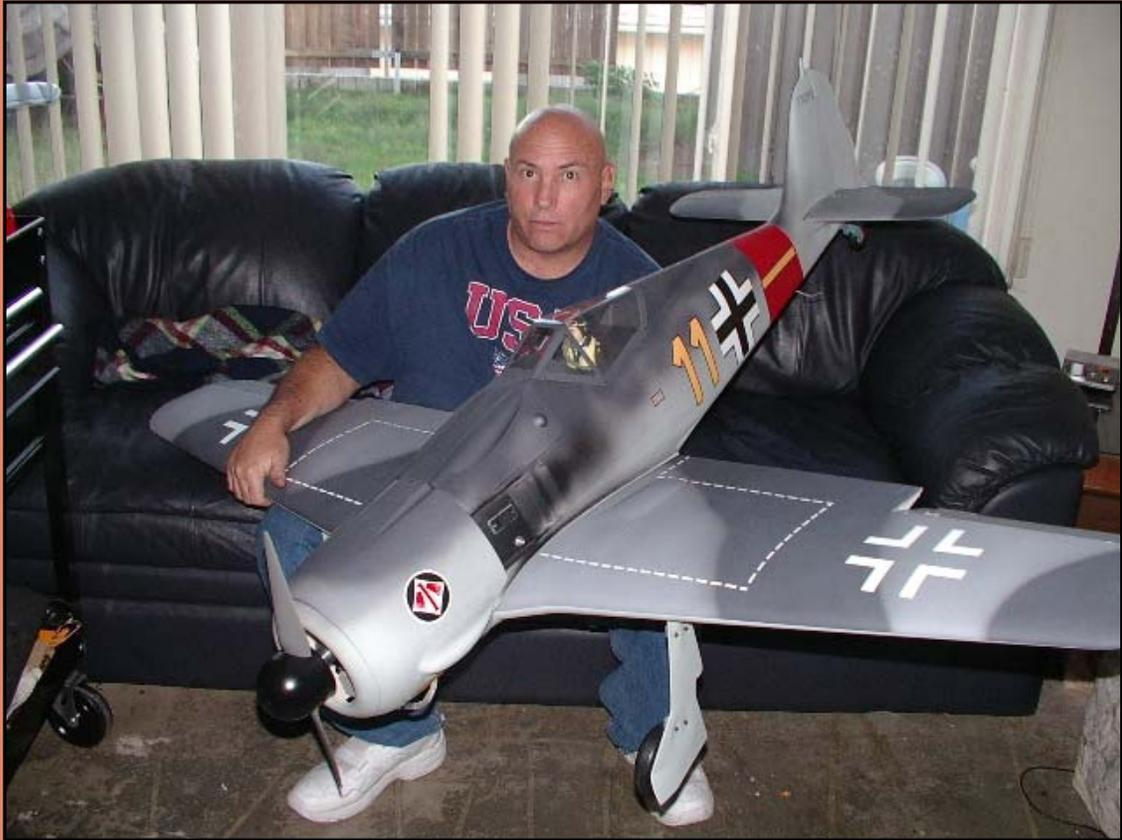
This model by Kondor Model Products has a wingspan of 71 inches, weighs a little over 17 pounds. It is powered by a Zenoah G-26 with electronic ignition, recently we have purchased a 3 bladed prop and spinner. The Kondors air retracts that were specially made for the FW-190 keep the airplane up and looking good. It has not flown yet, but I am planning on flying it soon after it gets checked over.
