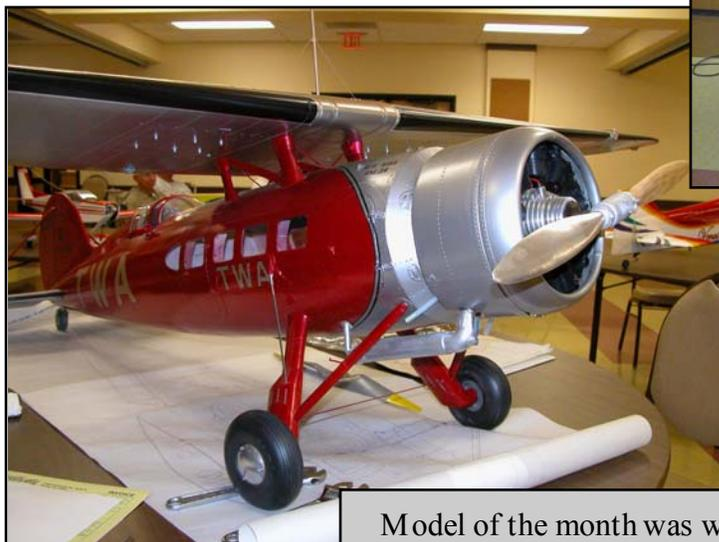
Model of the month was won by Ron Paterka, our expert scale modeler. His entry was a beautiful rendition of a Consolidated Fleetster of around 1934 vintage. The model was completely scratch built from a three-view drawing. It uses an RCV 1.20 engine with a scale appearing muffler for a totally enclosed installation.
